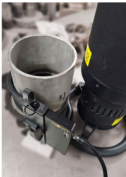
6 inch steel pipe, 6mm wall thickness, shot with YXLON ECO200DS
